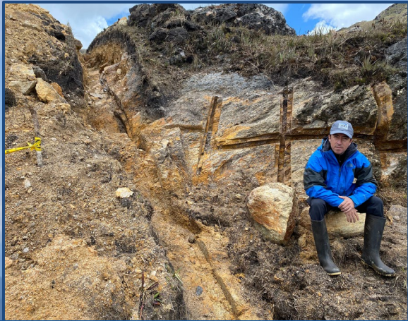
Country Manager, Santiago Yopez at Trench T-6 showing continuous channel sampling done with a rock saw; on the left are early exploration panel samples
